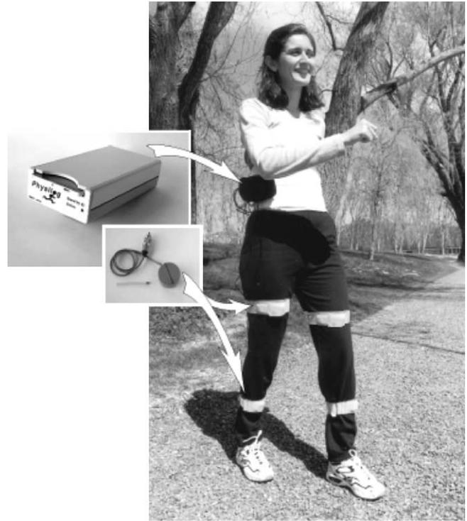
Fig. 1. A subject carrying the Physilog<sup>®</sup> system. The datalogger (300 g) can be fixed around the waist. Each sensor (gyroscope) is attached with elastic strip on each shank and thigh and linked with thin cable to the datalogger.
